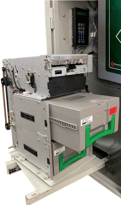
Rear Load machine above shown with optional **Patron Display with Attendant Key Switch** - displays Last 10 Transactions with Time & Date stamp with key switch.
